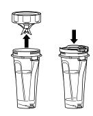
8 Turn cup over so blade assembly is on top. Rotate blade assembly counterclockwise to remove. To take your blended contents on the go, place the sealed spout lid on cup and turn clockwise to seal.
