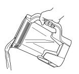
10 Unplug the unit when finished. To lift the motor base, place your hands underneath both sides of it and gently pull the unit up and toward you. Refer to the Care & Maintenance section for storing instructions.
