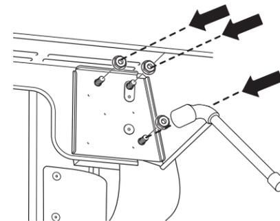
**IMPORTANT:** Screws must be fully tightened for stability.
