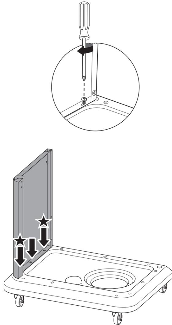
**IMPORTANT:** Screws must be fully tightened for stability.
