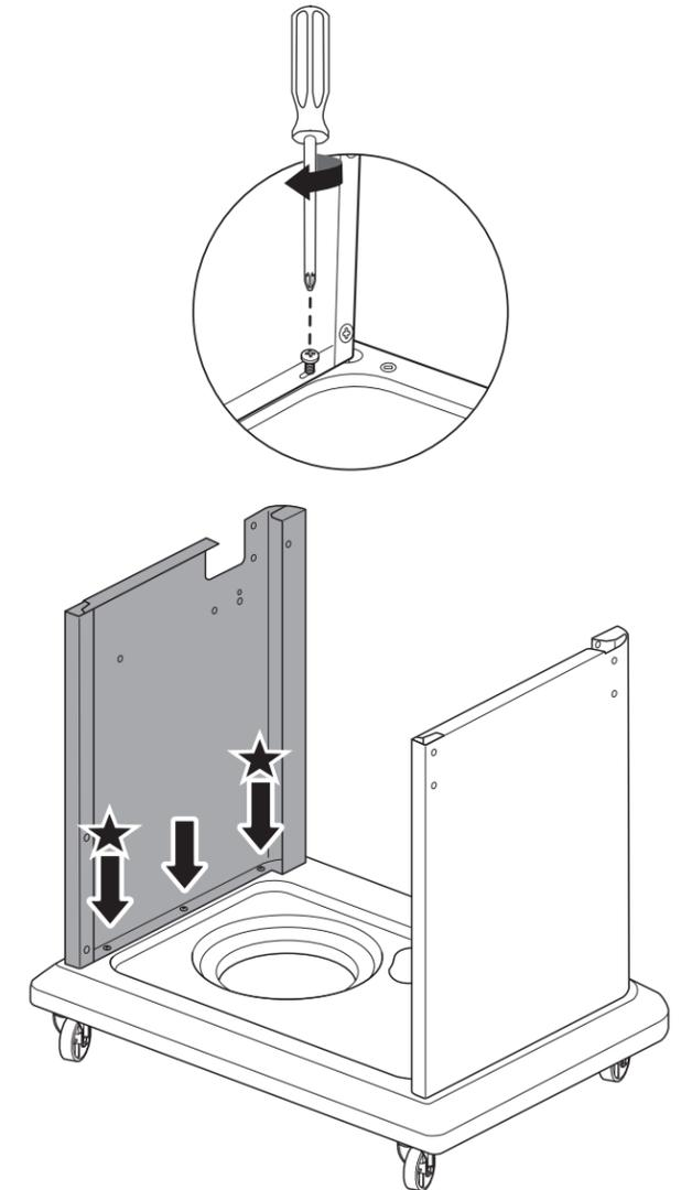
**IMPORTANT:** Screws must be fully tightened for stability.
