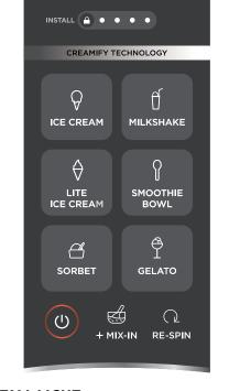
**INSTALL LIGHT** If the install light is blinking and the power light is solid, make sure the pint is properly installed, and the lid is fully secured. This can be verified by ensuring that the arrow on the processing lid is aligned with one of the arrows on the pint. If both the power light and install light are flashing, make sure the paddle is installed in the processing lid.
