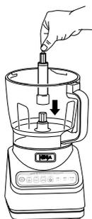
**2.** Install the disc spindle in the bowl.
