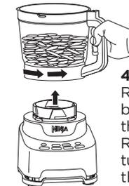
4. Remove the disc assembly by grasping the plastic grip, then remove the disc spindle. Remove bowl from base by turning it counterclockwise, then lifting it up.
