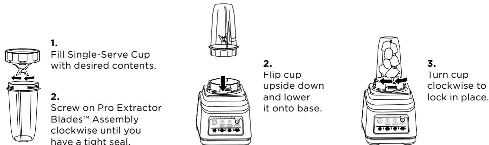
Once the Single-Serve Cup is locked onto base, press the Power button
