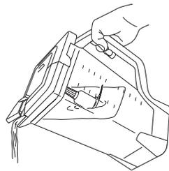
⚠ **CAUTION:** Blade Assemblies are not locked in place and are removable. If pouring with the lid removed, ALWAYS remove the Blade Assembly first.
