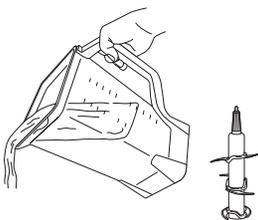
⚠ **CAUTION:** Blade assemblies are sharp, not locked in place and removable, handle with care. When handling the blade assemblies, always hold them by the shaft.
