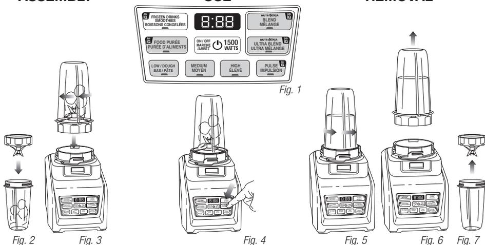
**NOTE:** Nutri Ninja™ | Ninja® Blender with Auto-iQ™ Technology can sense which jar is on the motor base. The available function lights will illuminate depending on which jar is placed on the motor base. (Fig. 1)
