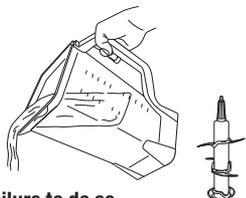
**▲ WARNING:** Chopping Blade Assembly is sharp and not locked in place. Before emptying contents carefully remove lid and Chopping Blade Assembly, holding it by the shaft. Failure to do so will result in a risk of laceration.
