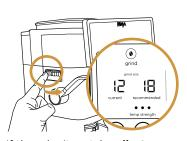
If they don't match, adjust current grind size by spinning the grind dial on left side of machine until it matches the recommended setting.
