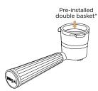
Locate your portafilter and ensure the double basket is installed.\*
