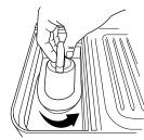
**4** Remove upper burr by rotating counterclockwise, aligning the orange arrow on the burr grinder with the orange arrow labeled ALIGN on the machine. Once aligned, lift upper burr out.
