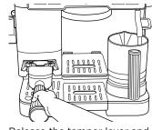
Release the tamper lever and remove the portafilter from the grinding cradle.
