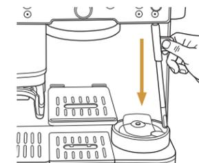
Push steam wand into its down position. The machine will automatically purge to clean inside of wand.
