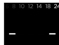
If your control panel is flashing each size, this means either there are grounds built up inside the top needle or calcium scale buildup in the brew system.
