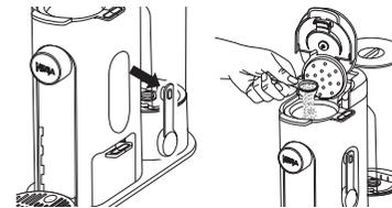
**NOTE: DO NOT** place ground coffee directly in the brew basket without the Permanent Filter installed.
