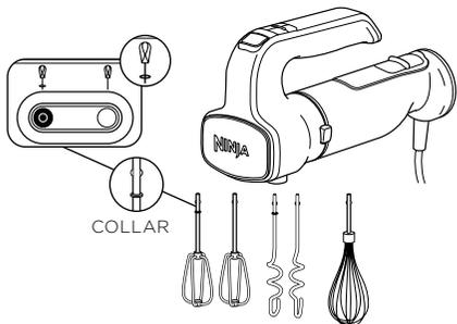
2 Attach both beaters, dough hooks, or the whisk using the accessory slots on the mixer head. Insert the beater or dough hook with the collar into the slot with the diagram showing a collar. The whisk can be inserted into either slot. You will hear a slight click when locked in place.
