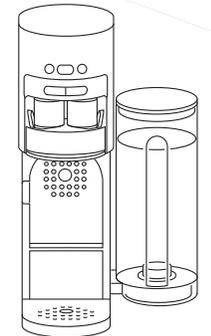
Flip Flavour Carriage up into the closed position. An error beep will be heard if the Flavour Carriage is not fully closed.
