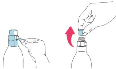
Remove the tamper seal and plastic cap from the top of the CO<sub>2</sub> canister.
