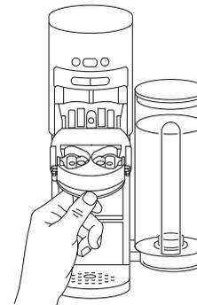
Open the Flavour Carriage by pressing down on the Mixing Chamber.
