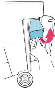
Open the CO<sub>2</sub> Door (remove instructional insert if not needed) and pull out the CO<sub>2</sub> collar.
