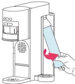
Install canister into collar by twisting to the right. **TWIST UNTIL TIGHT.**
