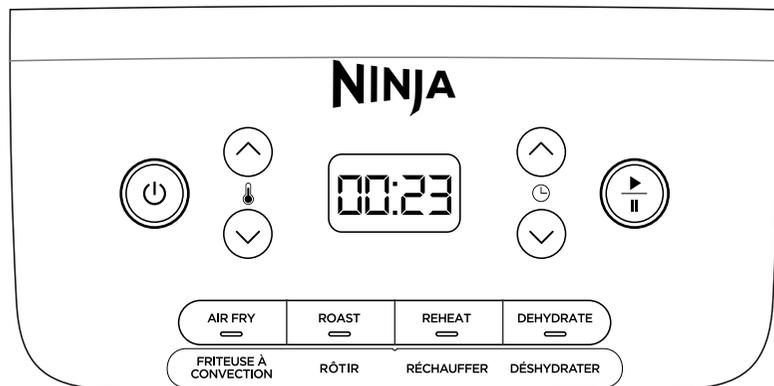
When setting time, the digital display shows HH:MM.
